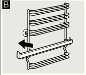
The rails only fit on the right or the left side. Ensure that, as shown in figure B, levels 1 and 2 are below and levels 3, 4 and 5 are above. The pull-out rail must be pulled out forwards.
